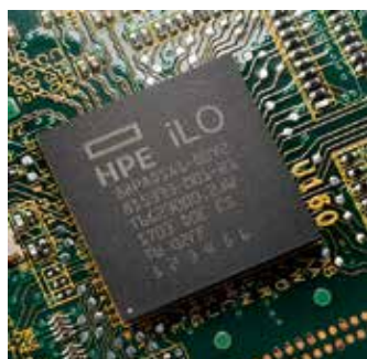
HPE Integrated Lights Out (iLO 5)
